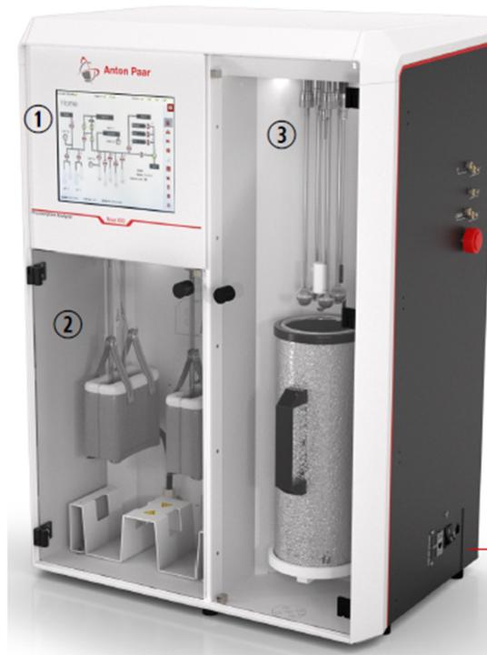
d. Load the sample cell on the degas station (②).
