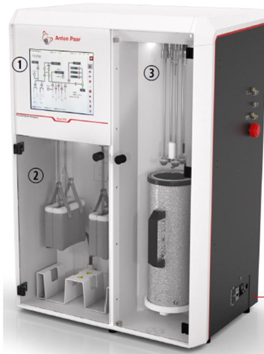
h. Load the sample cell on the degas station (②).
