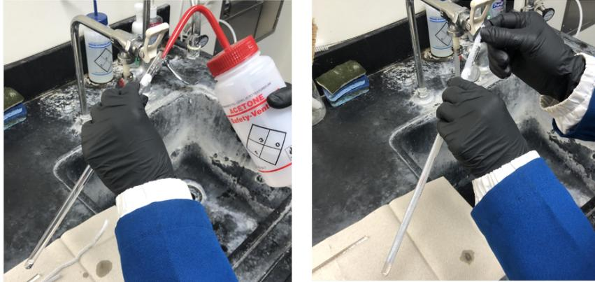
b.5. Clean up the rod in a such way. Wipe down with Kimwipes.
