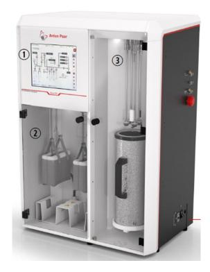
h. Load the sample cell on the degas station (2).
