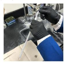
b.4. Clean up the cell with acetone by using a pipe brush. Repeat 1-2 times if needed.
