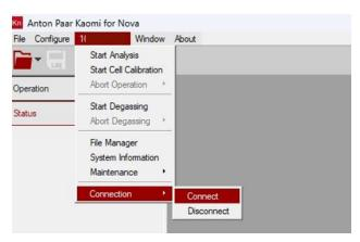
f. Connect with instrument. (S/N (1\*\*\*\*\*\*\*\*) > Connection > Connect)
