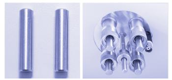
(left: image of 'dowel pins', right: as inserted in analysis stations)
