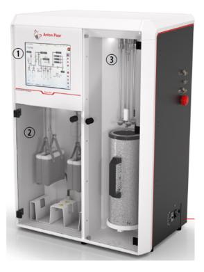
h. Load the sample cell on the degas station (2).
