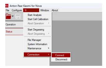
f. Connect with instrument. (S/N (1\*\*\*\*\*\*\*\*) > Connection > Connect)
