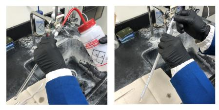
b.5. Clean up the rod in a such way. Wipe down with Kimwipes.
