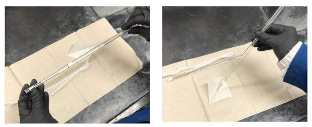
b.3. Clean up the cell with deionized water by using a pipe brush. Repeat 3-4 times if needed.
