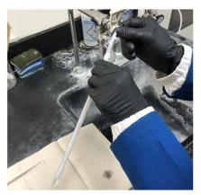
b.4. Clean up the cell with acetone by using a pipe brush. Repeat 1-2 times if needed.
