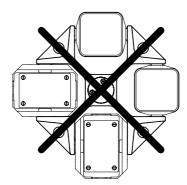
Fig. 6: Not allowed, because the pegs are not evenly loades, rotor is asymmetrically loades
