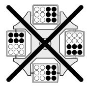
Fig. 8: Not permitted: pivots are not stressed evenly, rotor is not symmetrically loaded
